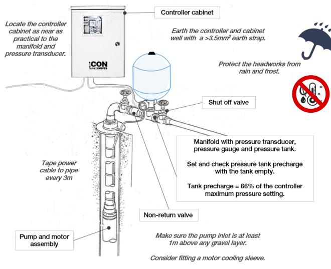
Set the pump a minimum of 1m below the well water level (drawdown level) when the pump is running.
