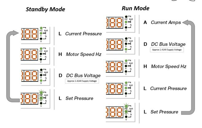
The operating set point pressure can be altered at any time using the UP and DOWN buttons. Any changes in this manner are not saved to parameter b00.01 <u>unless</u> <u>DATA/ENTER</u> is pressed to lock in the change.
